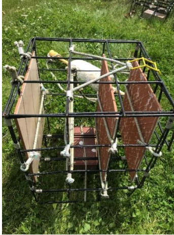
Figure 35. Recruitment device used in 2019 and 2020. Each device contains 4 tiles and is held in place with bricks and attached to a buoy.
